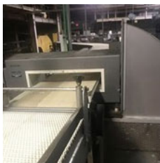
J-conveyor Discharge and Kwik Lok Tier
